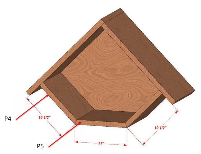
Attach front panels to back and top panels. Use 2" screws or nails.
