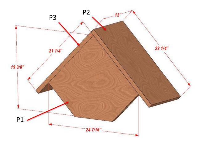
Attach top panels to back panel. Use 2" screws or nails.
