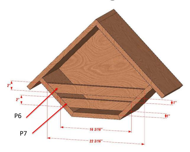
Add lintels to the front. Use 2" screws or nails.
